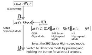
When used with the factory settings (Detection function: STND Standard mode) and the unit is subject to movement or vibration, the average value of the movement per 1 ms is displayed, so the indication may be displayed in 0.1 µm units. However, this is not the actual measurement value
